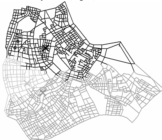
Fig. 2: The Network Voronoi diagram for the same three generators as in Figure 1, calculated on walking times along the street network.
